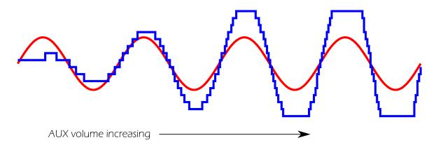
When the external input mixes with the square waves of the two oscillator voices, it will generally sound quieter. That is partially because square waves have high energy. To get an even mix, try turning down the oscillator voices or distorting the input by cranking the AUX volume knob.
