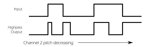
The key word is "attempts." In practice each edge on channel 1 inverts the output, and each edge on channel 2 sends it low. The resulting interference patterns resemble PWM. If channels 1 and 2 are tuned closely together, octaves form.
