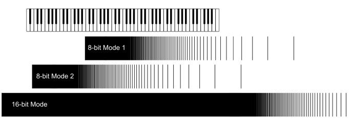
Switching between the two 8-bit pitch modes is done via back panel jumpers.
