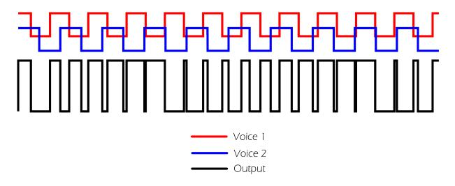
The POKEY chip highpass always uses the equivalent of a square wave from channel 2, so the wave setting of voice 2 does not impact filtering.
