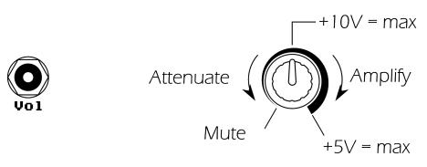
Turning clockwise amplifies the input, so it takes a lower input voltage to be max volume
